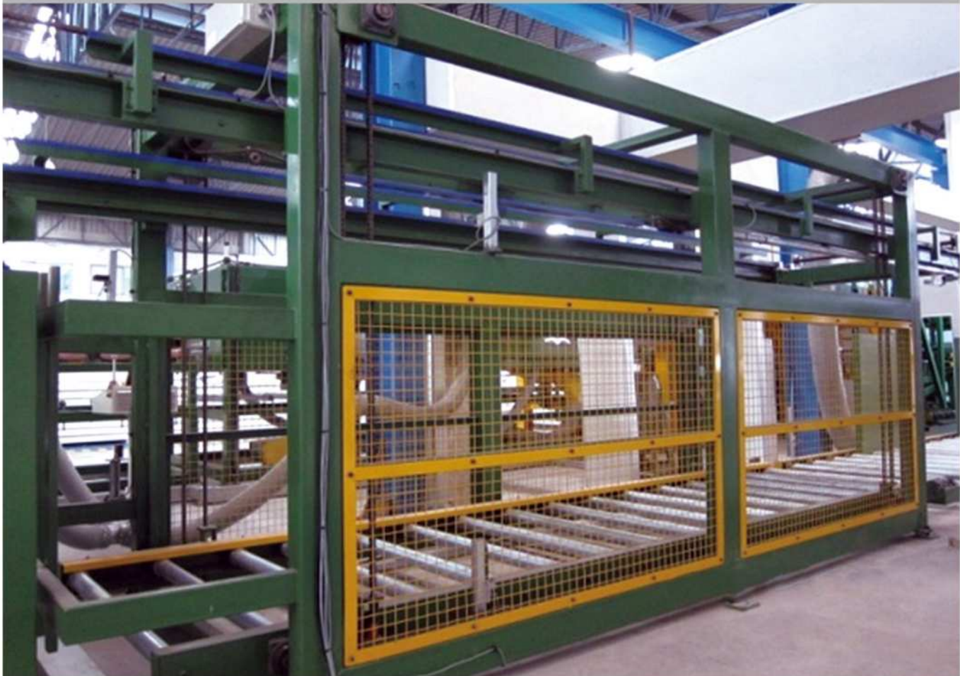
EPS board storage and supplying device
