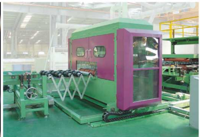
Panel cutting machine for EPS sandwich panel
