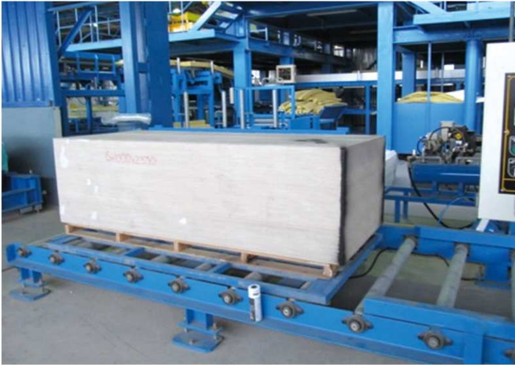
Cement board (or OSB) handling system
