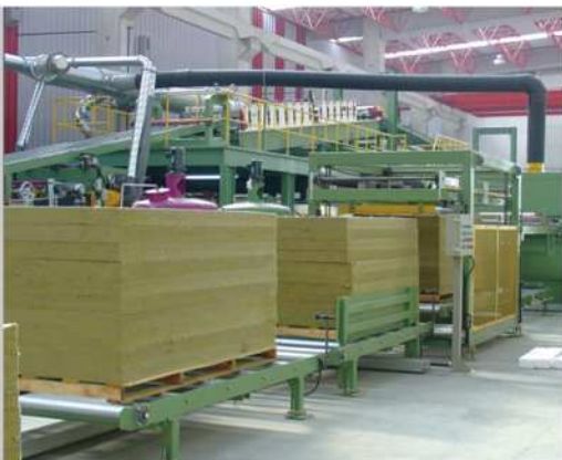
Mineral wool board supplying system
