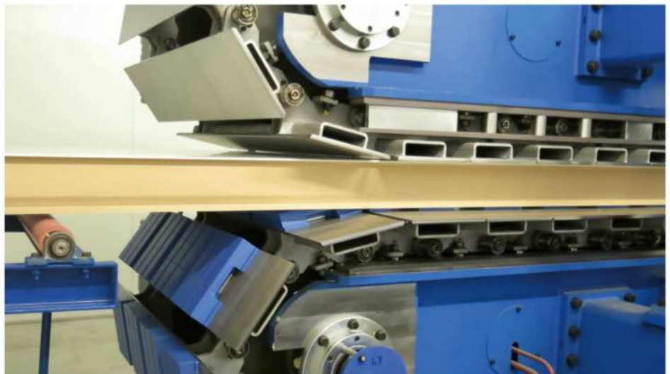
Double belt system for laminating with support block
